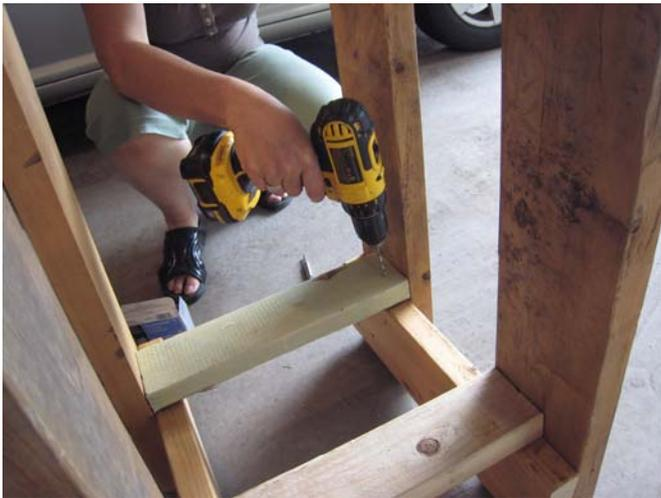
**5. Screw the bottom widthwise crosspieces onto the other crosspieces.**
