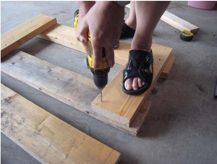
**3. Screw the crosspieces in place.** We used 2.5" screws, 4 on each end (16 total per side, 32 for both sides). We drilled holes before we drilled the screws so that the wood wouldn't crack.
